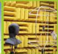
Semi-anechoic chamber According ISO 3744 According ISO 3745 According ISO 3746
